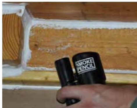
All Options: Test with smoke pencil to verify no air movement
